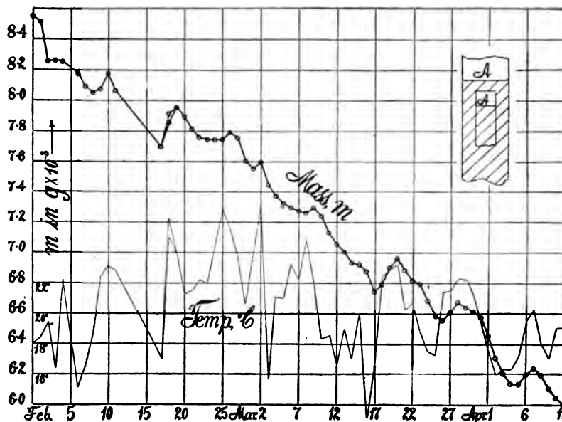
FIG. 6.—Loss of mass of gas in diver in lapse of days. Diffusion of air into air.
